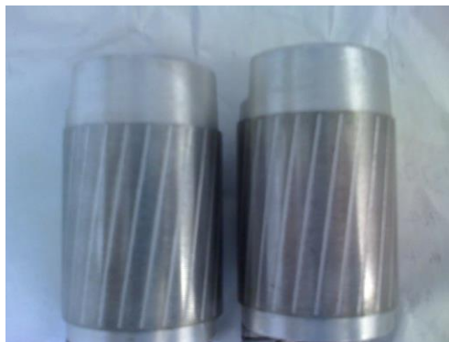
Figure 2: Rotor after cleaning with hydrocarbon agent (AHC-04)
