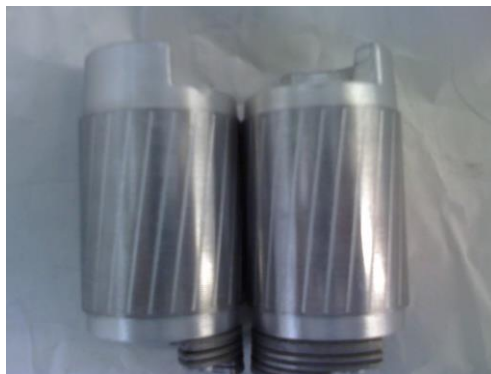
Figure 1: Rotor after cleaning with hydrocarbon agent (AHC-33P)
