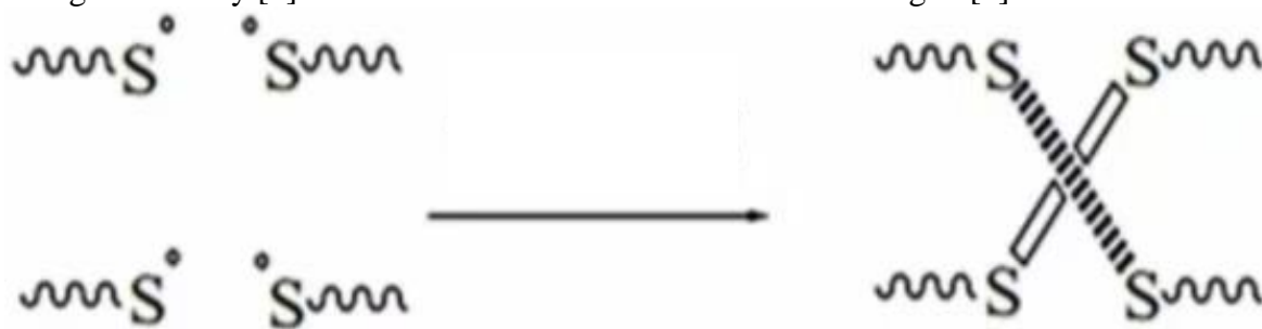
Figure 2 Schematic diagram of the principle of disulfide bond self-repair performance.
