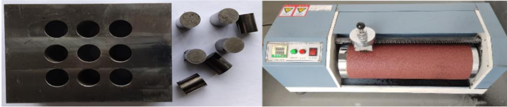
Figure 3: DIN Abrasion Tester Sample Preparation Mold and Actual Product Image
