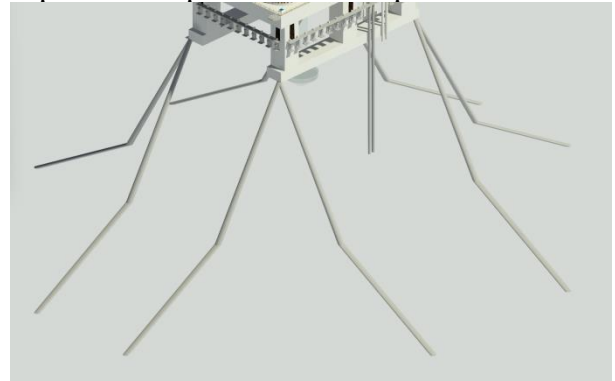
Figure 2: Catenary mooring device
