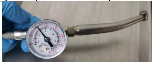
Figure 1: Pressure testing of hand pieces
