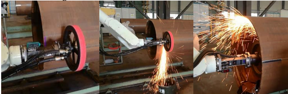
Figure 5: Engineering Application of Intelligent Grinding Robot for Welding Seam of Welded Pipe
