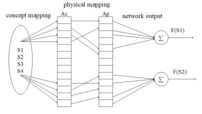
Figure 1: Topological structure of CMAC
