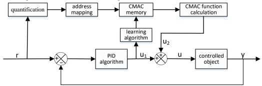
Figure 3: Structure of CMAC-PID controller
