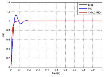
Figure 4: Comparison between CMAC-PID controller and traditional PID controller
