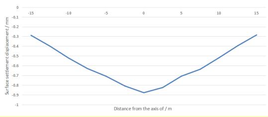
Numerical simulations of lateral surface subsidence
