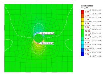
Figure 7: Vertical displacement cloud map of 12m tunneling
