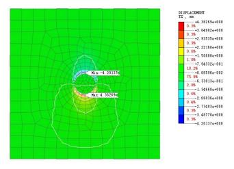
Figure 6: Vertical displacement cloud map of 8m tunneling
