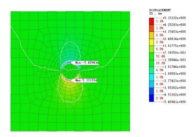
Figure 8: Vertical displacement cloud map of 16m tunneling
