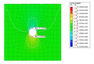
Figure 9: Vertical displacement cloud map of 20m tunneling
