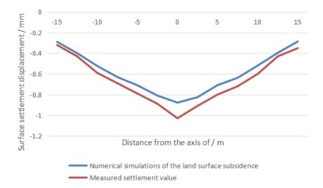
Figure 4: Comparison of simulated values and measured values of surface subsidence
