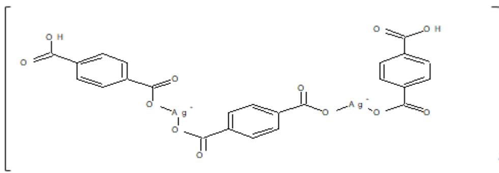
Figure 1: Ag-MOF conceivable bonding and repeating units.
