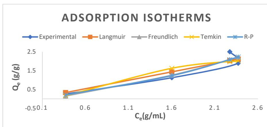
Figure 11: Isotherm plots for the adsorption of crude oil by Ag-MOF
