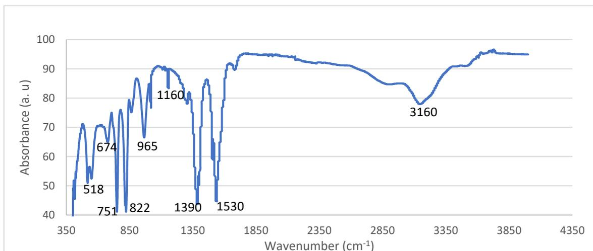
Figure 3: FTIR spectrum for bezene-1,4-dicarboxylic acid.
