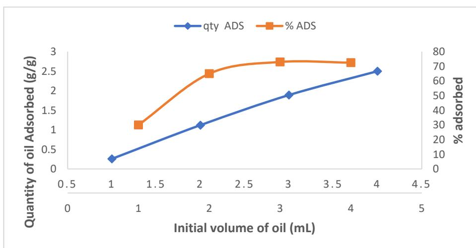
Figure 10: Effect of initial volume of crude oil on the quantity of oil adsorbed by Ag-MOF
