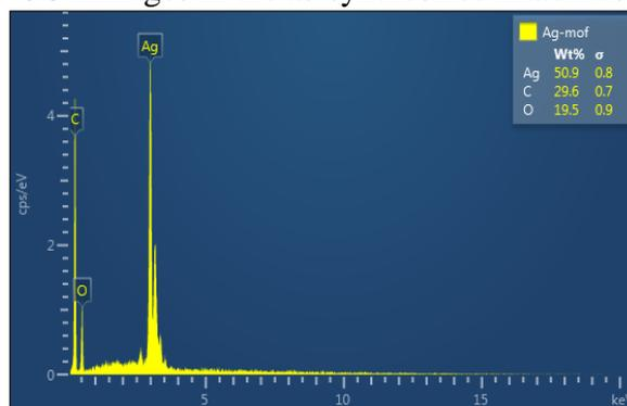
Figure 5: Benzene-1,4-dicarboxylic acid (BDA) (Terephthalic Acid) Linker of Silver Metal Organic Framework (Ag-MOF) using Energy Dispersive X-ray Spectroscopy (EDX).
