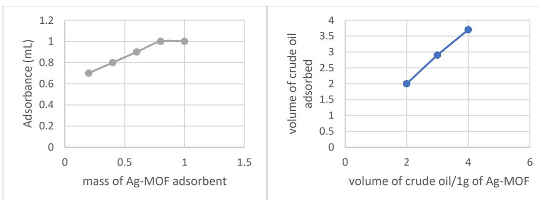
Figure 6: Effect of adsorbent dosage on the Adsorption of crude oil by Ag-MOF. And Figure 7: Volume of Crude oil in (mL)/1g of Ag-MOF respectively given above.
