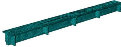
Figure 3: Mesh Generation of 30m Segmental Prefabricated t-Beam
