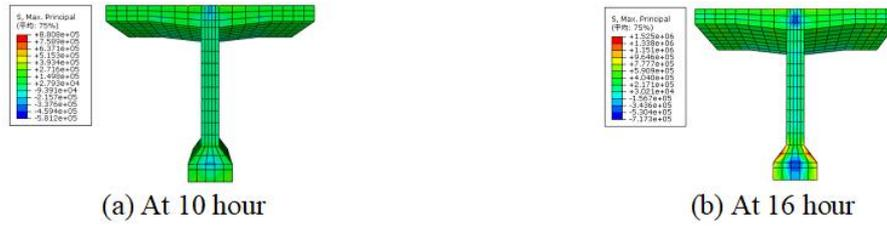
Figure 6: Maximum Principal Stress of t-Beam
