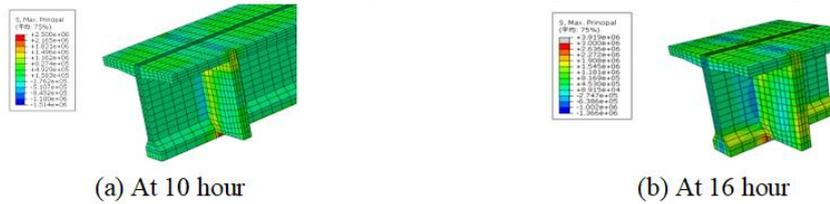
Figure 7: Maximum Principal Stress of Diaphragm
