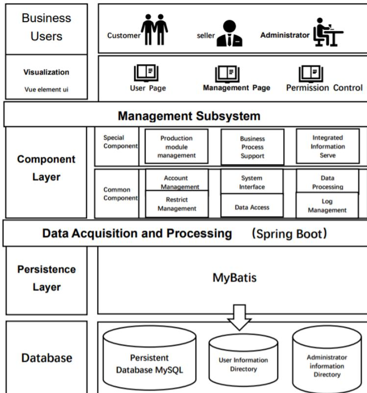
Figure 2: server system architecture
