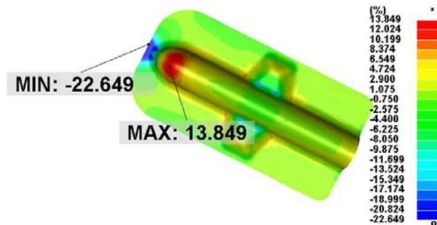
Figure. 12 Cloud chart of second order thinning rate of parts
