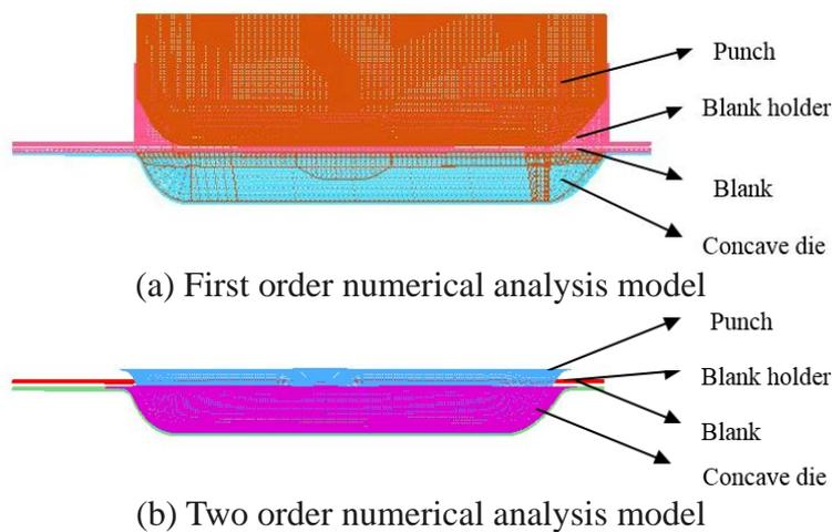
Figure. 6 Numerical analysis model
