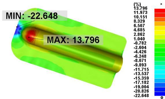
Figure. 10 Cloud chart of first order thinning rate of parts
