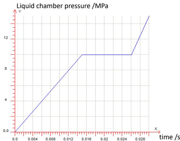
Figure. 7 Pressure loading curve of liquid chamber
