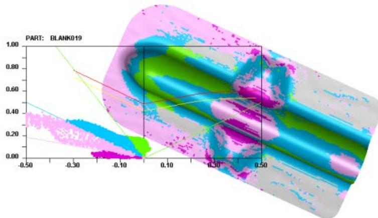
Figure. 11 Part secondary forming limit diagram (FLD)
