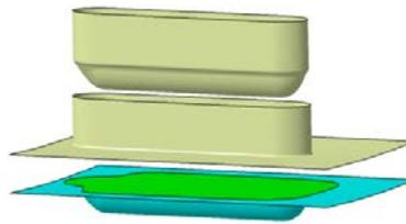
*Figure. 2 Finite element model of first order forming*
