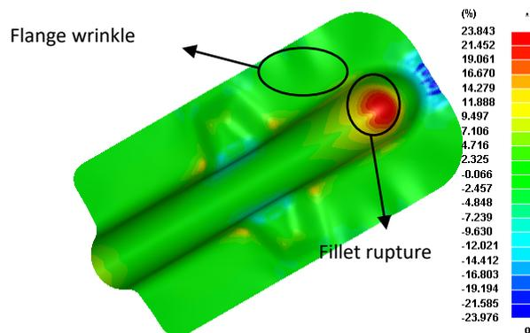
Figure. 5 Numerical analysis of rigid drawing
