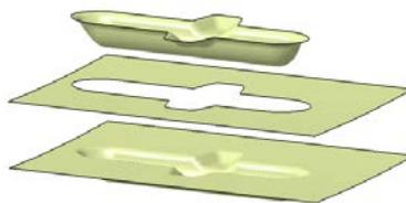
*Figure. 3 Finite element model of second order forming*
