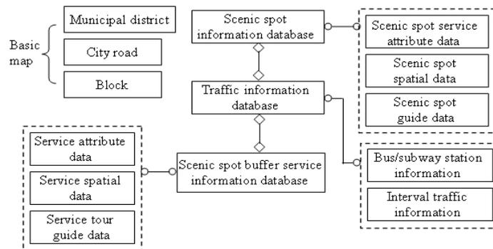
Fig. 4 System data model design
