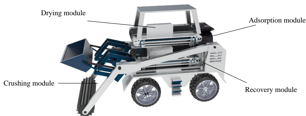
Figure 3: Schematic diagram of the overall device mechanism
